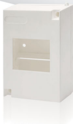
name N 2 A type IP 40 □ In 63A dimensions 130 x 87 x 57 number of modules 3 + 1 PE, N terminal -
