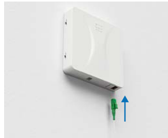
Latch on on the cover and plug the patch cable in to the router (optional).
