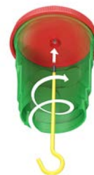
M5 metal nut for secure mounting of light hooks up to 100 N (10 kg) according to DIN EN 60670.
