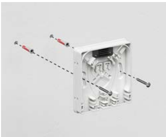
Create 5 mm drill holes.
