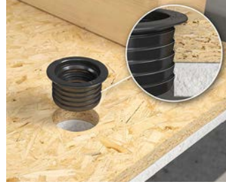
Fixing the wall connection element through the peripheral sealing ribs in the wall boarding.
