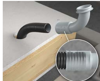
The protruding electrical installation conduit is inserted into the conduit holder of the 90° bend up to the depth stop and locked in place.
