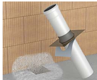
Pull the sleeve over the cable/conduit and remove the protective foil.
