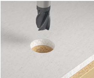
Machine creation of the exact installation opening of Ø 38 mm.
